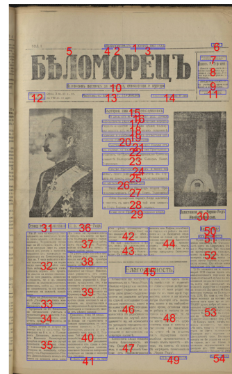
Figure 2: An example of a page where the blocks are ordered with the help of the reading order algorithm. The resulting order is consistent with both — the five-column layout and the partial horizontal separator.
