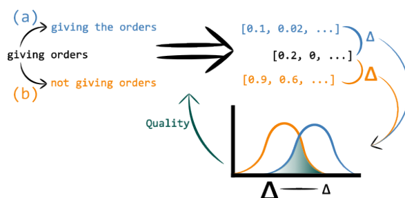
Figure 1: Concept Separation Curves. This example has been translated from the Dutch sentence "bevelen geven" (giving orders), which originates from the CompetentNL dataset. Initially, a set of perturbations is computed for a given sentence: a) surface-level perturbation, and b) semantic change. Following the process of embedding each sentence, the difference per vector is measured. The application of this process to the entire corpus provides insight into the quality of the embedding, as demonstrated by the overlap between the curves.
