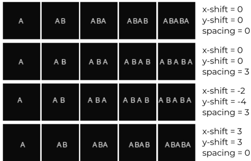
Figure A.1: Examples from the generated dataset and model training. All the images are comprised by a string of 1 to 5 letters, using only the uppercase characters A and B. To generate variations of this strings the spacing and the x and y position were modified.
