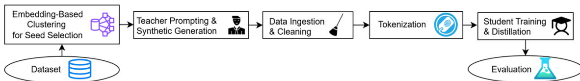
Figure 1: Overview of the proposed framework: clustering-based seed selection → GPT-4o prompting and synthetic generation → compact student fine-tuning and evaluation.
