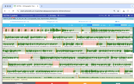
Figure 2: Automatically generated raw transcript in the 2D editor in Octra. Green transcription units contain transcript text, red ones are empty. Boundaries were set by whisperX. Some of these boundaries are so close to each other that they are visible only after zooming in (cf. Figure 5).
