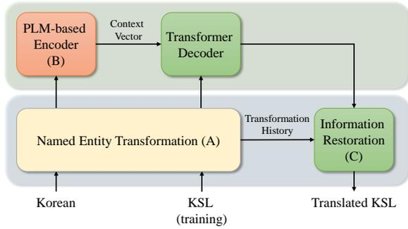
Figure 4: An overview of our SLT system. First, the named entity transformation module transforms input sentences (see (A)). Next, a PLM (e.g., BERT) encodes the transformed source sentences to context vectors (see (B)) and the decoder generates translated KSL sequences containing named entity tokens. Finally, the information restoration module converts named entity tokens to their original expressions using a transformation history (see (C)).
