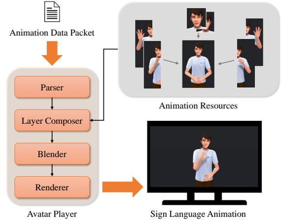
Figure 5: A high-level overview of our avatar player pipeline. The player parses the input data packet, composes animation layers based on each input channel, calculates animation timing and inter-animation blending data, and renders the avatar video.
