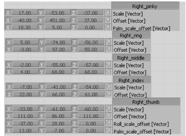
Figure 1: One user interface for manual calibration of two data gloves at a time. In the figure, only the half of the interface for the right hand is shown.
