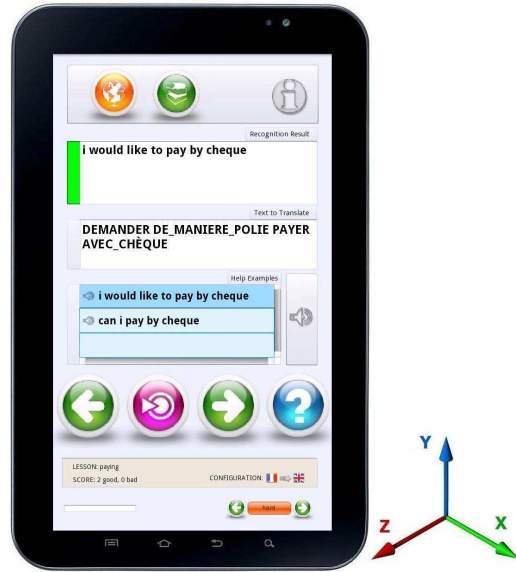
Figure 1: CALL-SLT application running on the Samsung Galaxy Tab. The middle pane shows the prompt; the top pane, the recognition result; the bottom pane, text help examples. Button controls are arranged along the bottom
