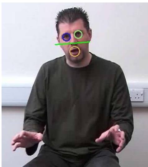
Figure 2: The Head tracker in action
