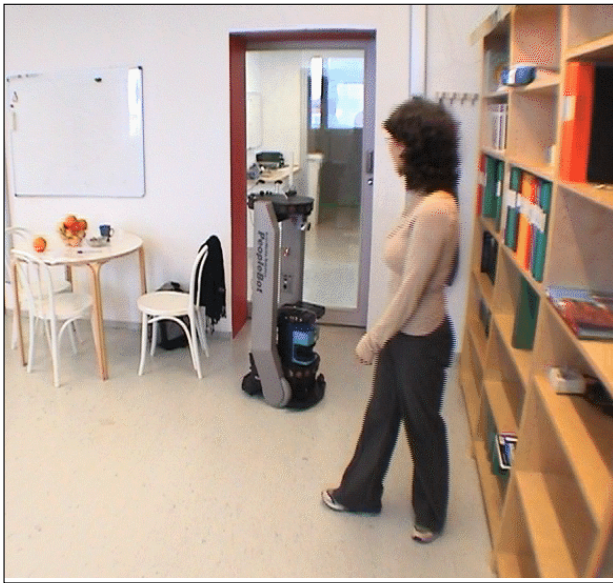
Figure 2: The modified ActivMedia PeopleBot used for the corpus collection and a user engaged in interaction.
