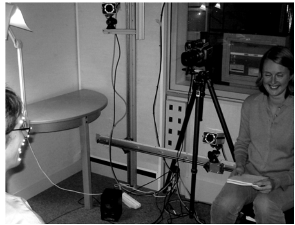
Figure 4 Data collection setup in corpus 1 with video and IR-cameras, microphone and a screen for prompts.
