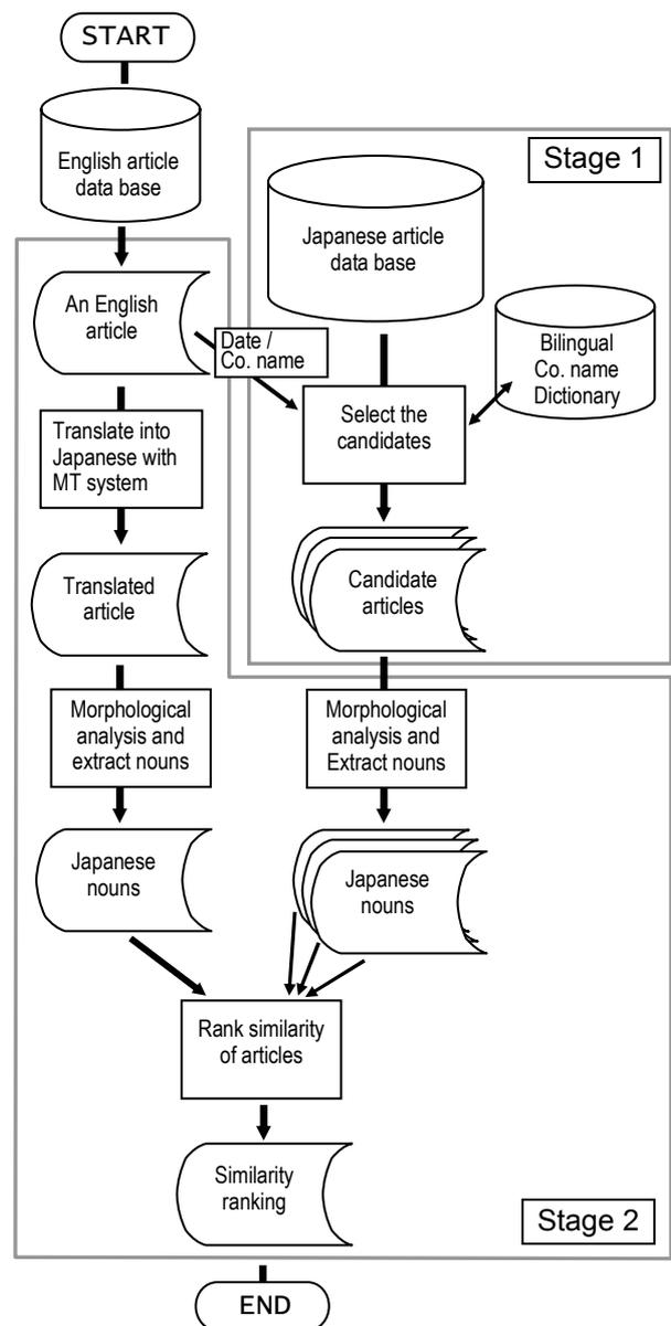
Figure 1: Alignment process
